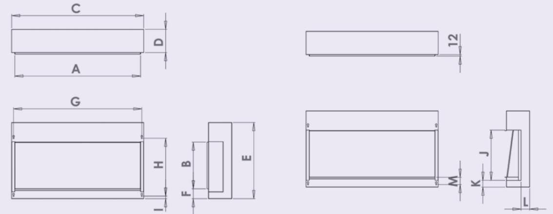
Shown as supplied for front opening arrangement with side panels in position either or both side panels can be removed to give a 2 sided or 3 sided arrangement
